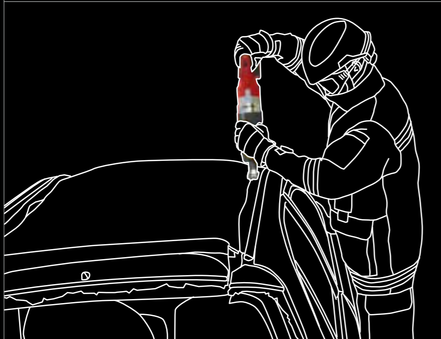
4 An rechter Dachreling entlang aufsägen Saw along right roof rack
