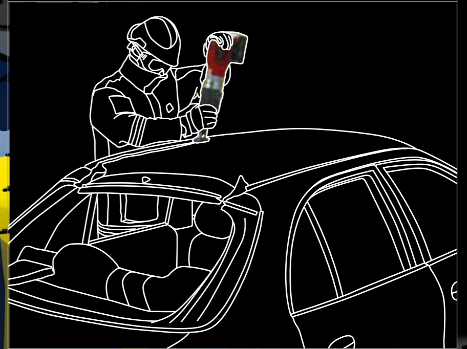
3 An linker Dachreling entlang aufsägen Saw along left roof rack
